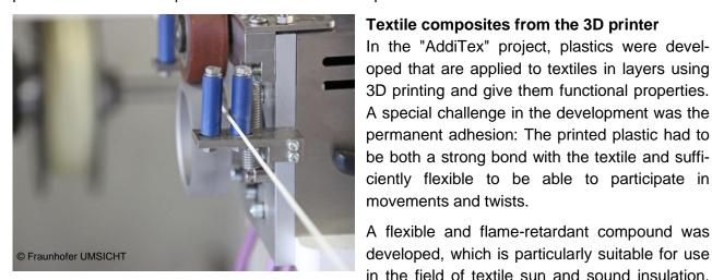
The new AddiTex compound comes out of the extruder as a filament for 3D printing.
