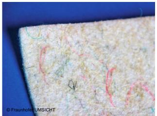
Prototype of a geotextile filter for bank protection.
