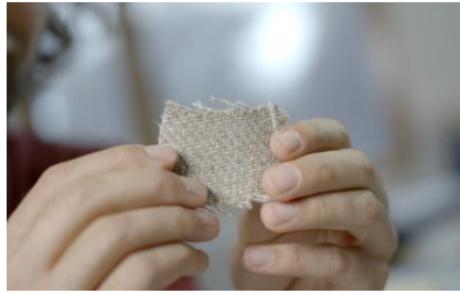
Textile made of flax fibers inserted into the board as reinforcement.
