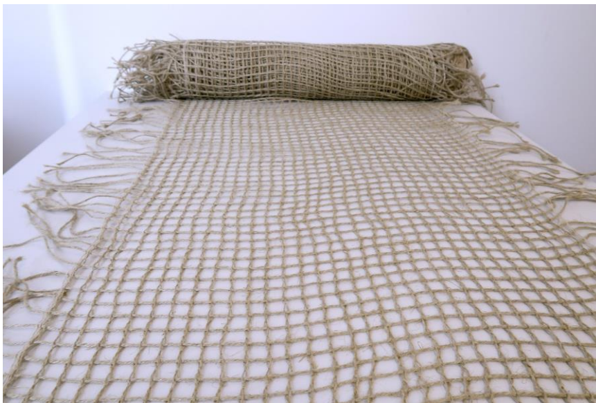
The renewable natural fibers used for the leno fabric - which are available regionally or Europe-wide - and a partially bio-based coating contribute towards improving the carbon footprint of the construction industry. (© WKI)
